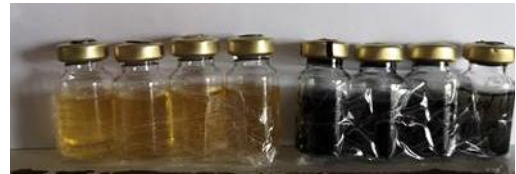
Microbiological contamination in the closed loop after 2 days of inoculation (Anaerobic Bacteria test – inoculated vials on the right side).
